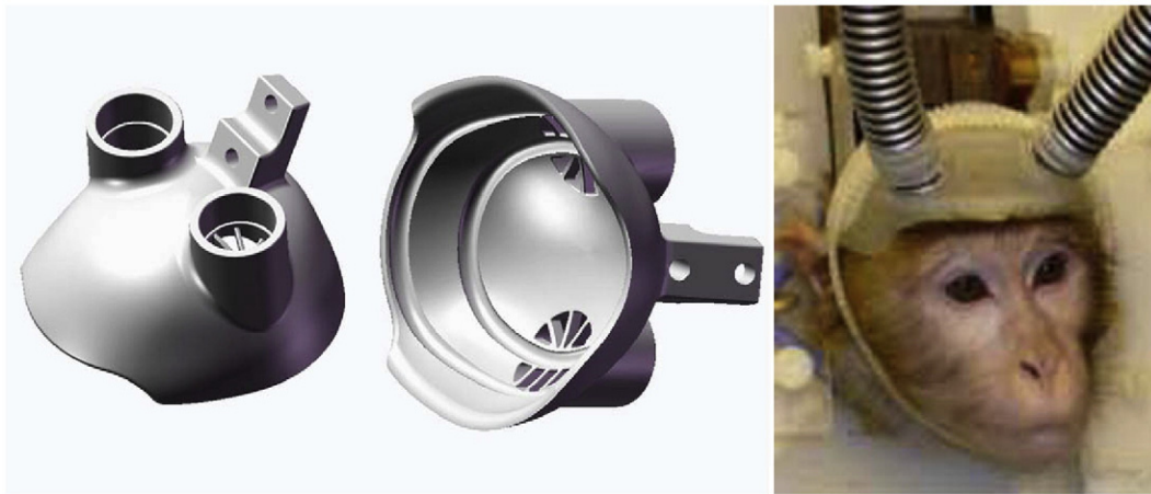
Fig. 1. (Left) The vacuum helmet and (right) an alert monkey sitting calmly, in the helmet, ready to be scanned.
